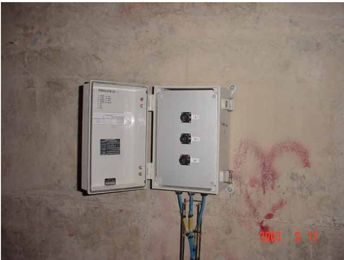
3 point measuring box for direct connection instrument-readout
