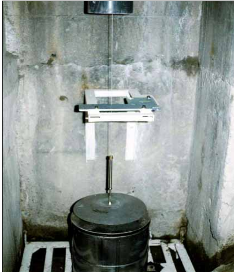
Direct pendulum with optical coordinate baseplate
