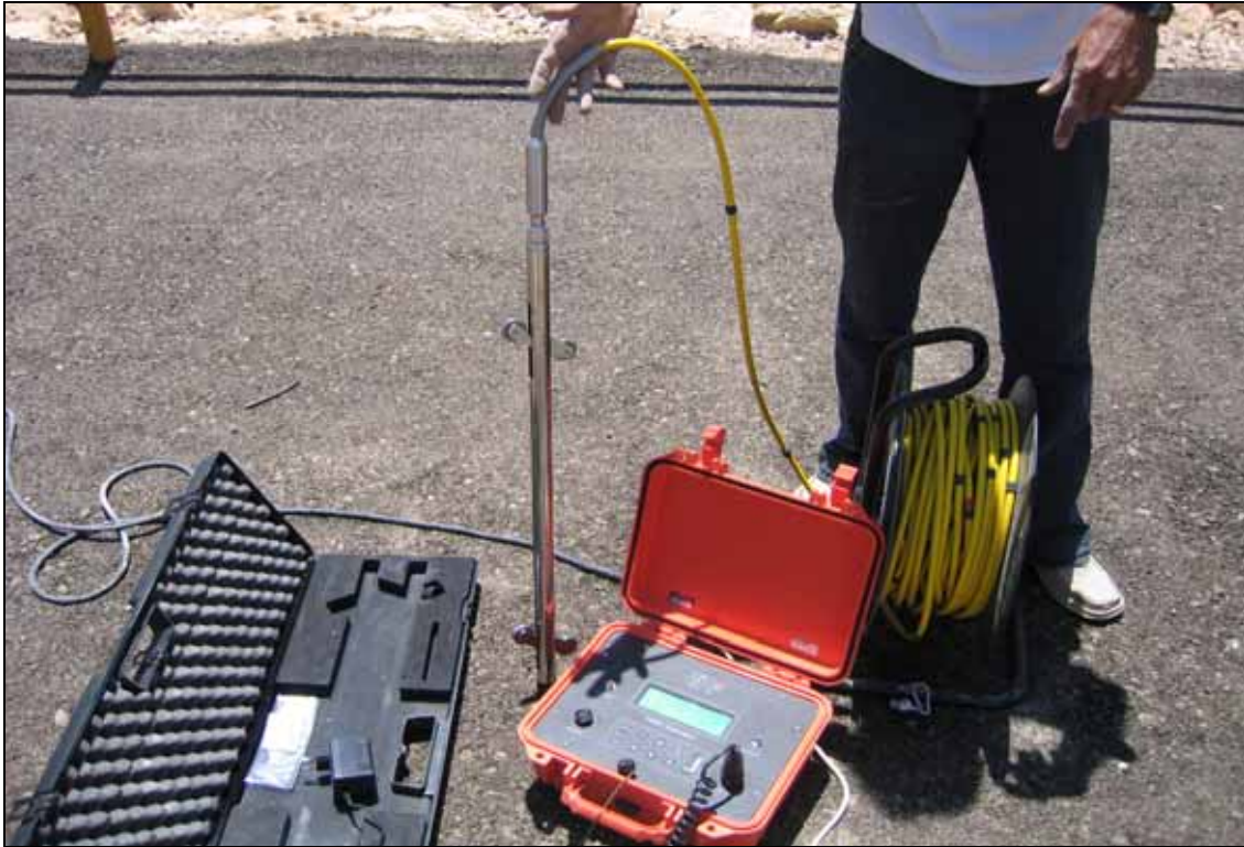
Inclinometer system ready for measurements
