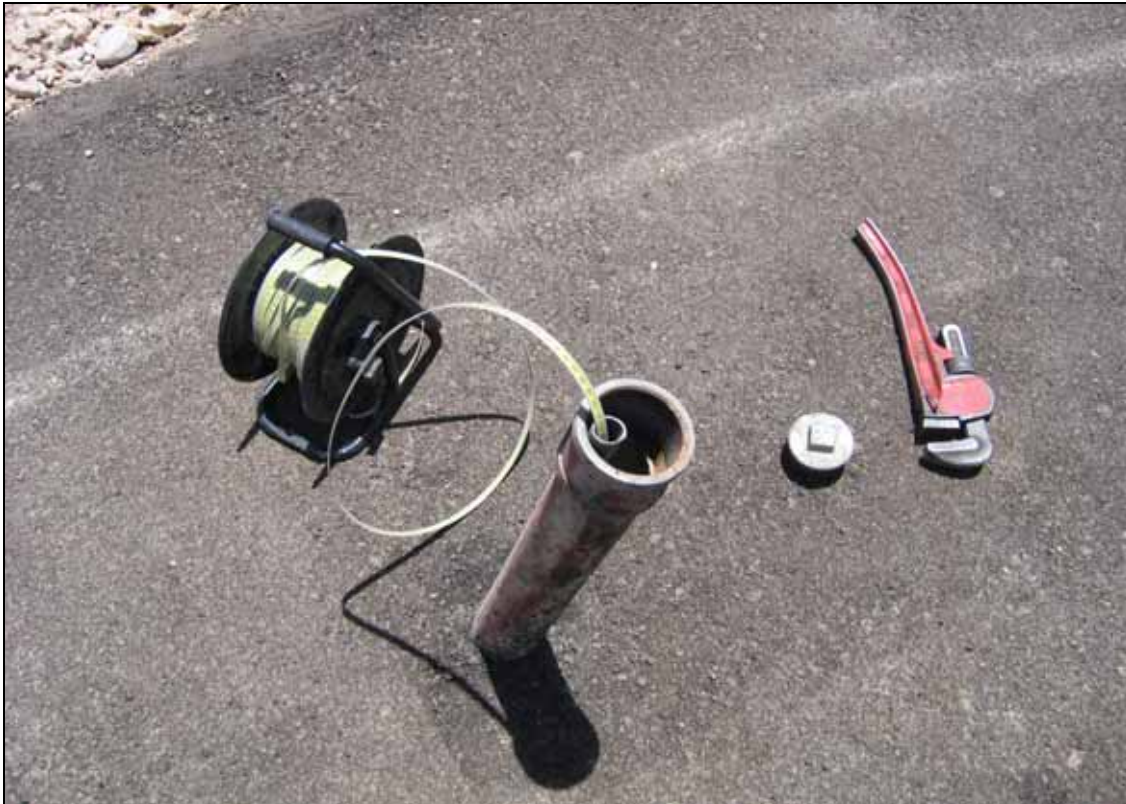
Water table measurement with water level indicator
